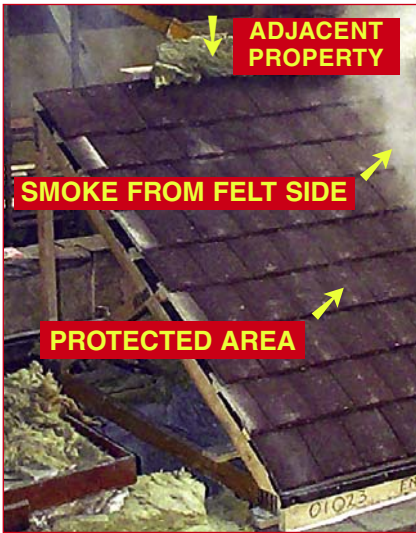
DURING THE FIRE TEST
